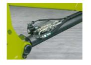
Thanks to electrical switching in the FL and FL C series, the safety valves can be combined with the SHOCK ELIMINATOR vibration damping system.
