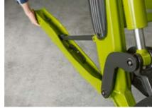
The support legs fold easily under the boom and do not obstruct the view of the front loader.
